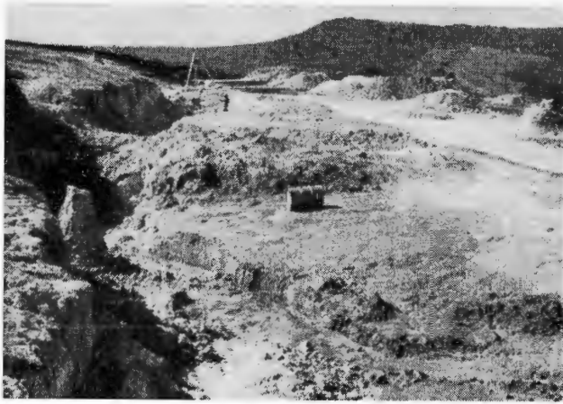
The Kaolin deposit at Mahlangatsha showing the quarry and the dumps of kaolin awaiting transport to railhead. The ore-body is vertical and is between 25 and 30 feet wide.
